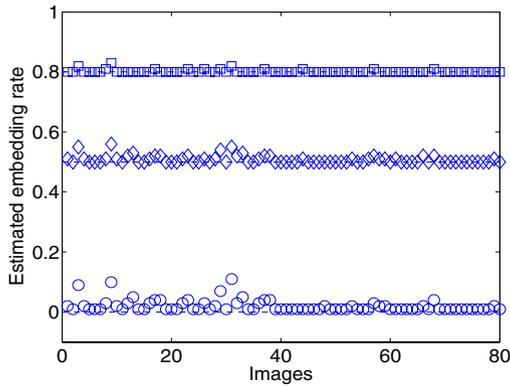
**Fig. 7.** Estimated embedding rates for the assignment steganography based on component sum (Circles: originals; Dimonds: stego-images with  $\alpha = 0.5$ ; Squares: stego-images with  $\alpha = 0.8$ )
